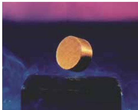
Figure 30.34 A small permanent magnet levitated above a disk of the superconductor \text{YBa}_2\text{Cu}_3\text{O}_7 cooled to liquid nitrogen temperature (77 K).
