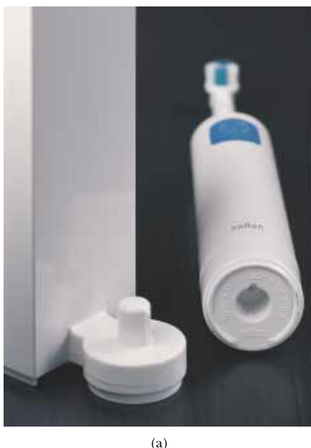
Figure 32.13 (a) This electric toothbrush uses the mutual induction of solenoids as part of its battery-charging system. (b) A coil of N_H turns wrapped around the center of a solenoid of N_B turns.
