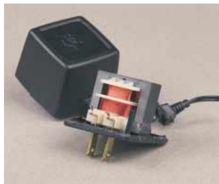
Figure 33.20 The primary winding in this transformer is directly attached to the prongs of the plug. The secondary winding is connected to the wire on the right, which runs to an electronic device. Many of these power-supply transformers also convert alternating current to direct current. (George Semple)
