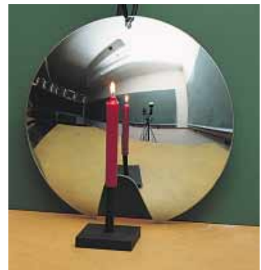
Figure 36.15 Ray diagrams for spherical mirrors, along with corresponding photographs of the images of candles. (a) When the object is located so that the center of curvature lies between the object and a concave mirror surface, the image is real, inverted, and reduced in size. (b) When the object is located between the focal point and a concave mirror surface, the image is virtual, upright, and enlarged. (c) When the object is in front of a convex mirror, the image is virtual, upright, and reduced in size.
