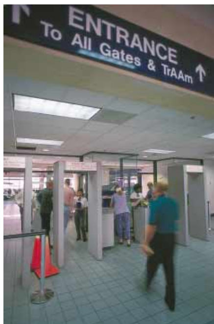
Figure 33.17 When you pass through a metal detector, you become part of a resonant circuit. As you step through the detector, the inductance of the circuit changes, and thus the current in the circuit changes. (Terry Qing/FPG International)
