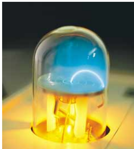
The blue-white arc in this photograph indicates the circular path followed by an electron beam moving in a magnetic field. The vessel contains gas at very low pressure, and the beam is made visible as the electrons collide with the gas atoms, which then emit visible light. The magnetic field is produced by two coils (not shown). The apparatus can be used to measure the ratio e/m_e for the electron.
