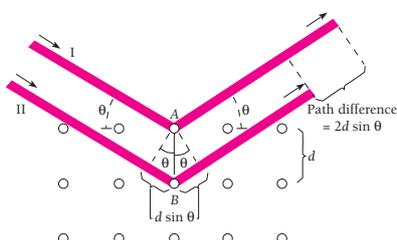
Figure 2.20 X-ray scattering from a cubic crystal.
