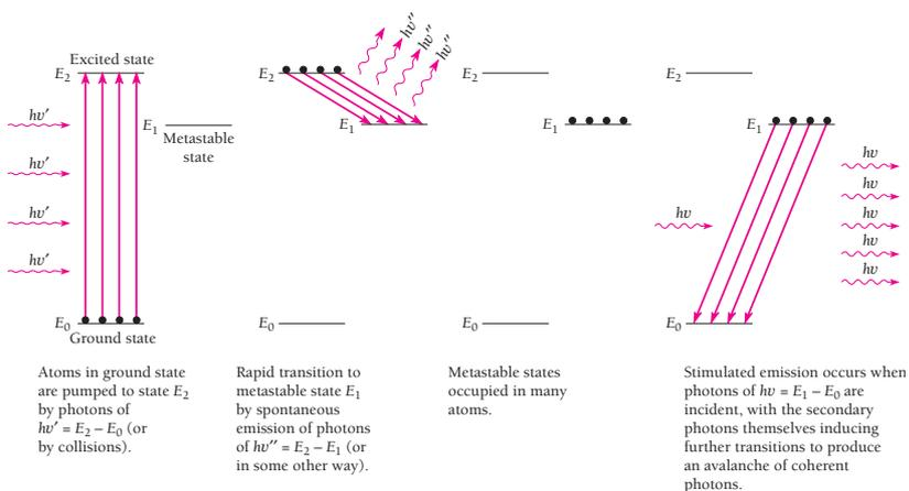
Figure 4.26 The principle of the laser.
