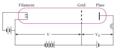
Figure 4.21 Apparatus for the Franck-Hertz experiment.
