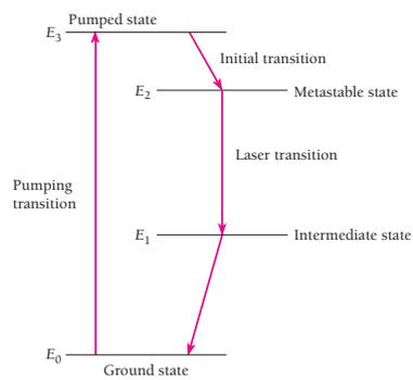
Figure 4.28 A four-level laser.
