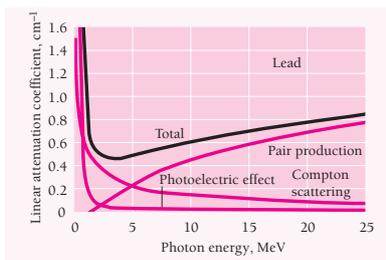
Figure 2.29 Linear attenuation coefficients for photons in lead.
