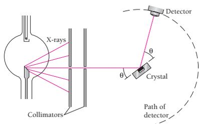
Figure 2.21 X-ray spectrometer.
