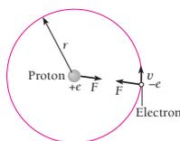
Figure 4.5 Force balance in the hydrogen atom.
