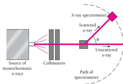
Figure 2.23 Experimental demonstration of the Compton effect.
