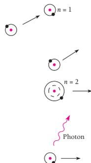
**Figure 4.18** Excitation by collision. Some of the available energy is absorbed by one of the atoms, which goes into an excited energy state. The atom then emits a photon in returning to its ground (normal) state.
