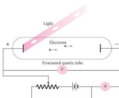
Figure 2.9 Experimental observation of the photoelectric effect.
