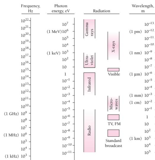
Figure 2.2 The spectrum of electromagnetic radiation.
