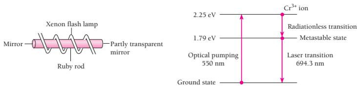
Figure 4.27 The ruby laser. In order for stimulated emission to exceed stimulated absorption, more than half the  $Cr^{3+}$  ions in the ruby rod must be in the metastable state. This laser produces a pulse of red light after each flash of the lamp.
