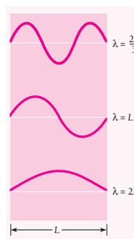
**Figure 2.7** Em radiation in a cavity whose walls are perfect reflectors consists of standing waves that have nodes at the walls, which restricts their possible wavelengths. Shown are three possible wavelengths when the distance between opposite walls is  $L$ .
