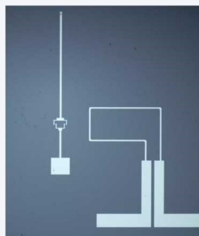
A transmon qubit designed for 3D cavity architecture with a fast-flux line.
