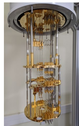
Dilution refrigerator, where the physical qubits are placed PC: Prof. Baladitya Suri
