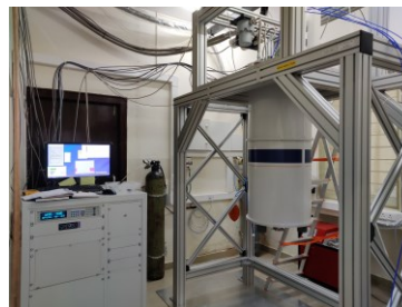
Dilution refrigerator, where the physical qubits are placed PC: Prof. Baladitya Suri
